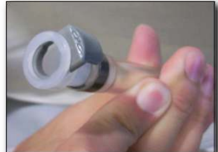
Inspect Connector on End of Hose for Damage
