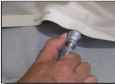
Push in Grey Tab Where Hose Attaches to Air Chamber & Remove Hose
