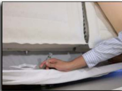
Push in Grey Tab on Air Hose Where It Connects to Air Chamber And Remove Hose
