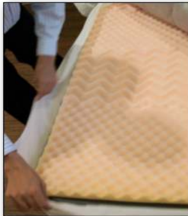
Position Foam Over Chamber & Cover with Border Wrap
